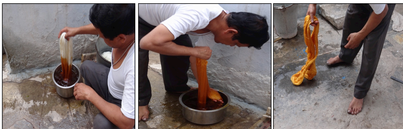
a. Yarns dipped in cold dye bath
