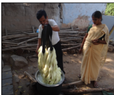
b. Silk yarns immersed in degumming solution
