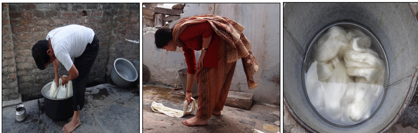
a. Yarns squeezed and beaten on floor two-three times
