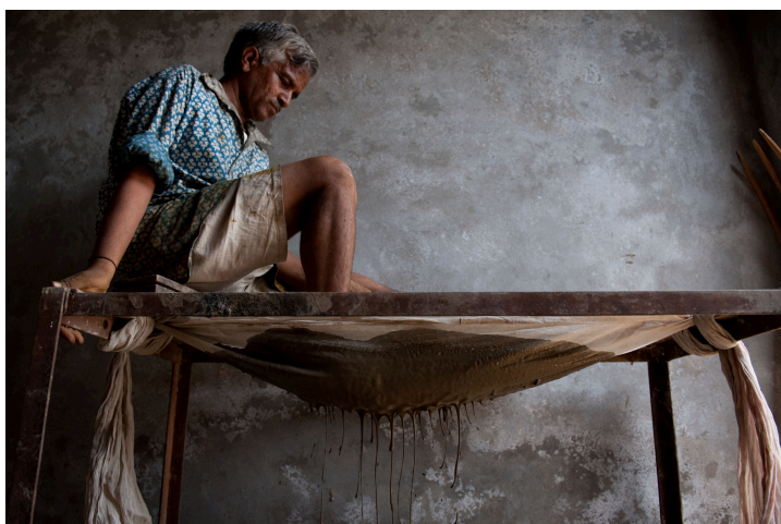
Figure 4: Suraj Narayan Titanwala straining dabu (mud resist paste) through a fine muslin cloth. . Photo Courtesy: Author
